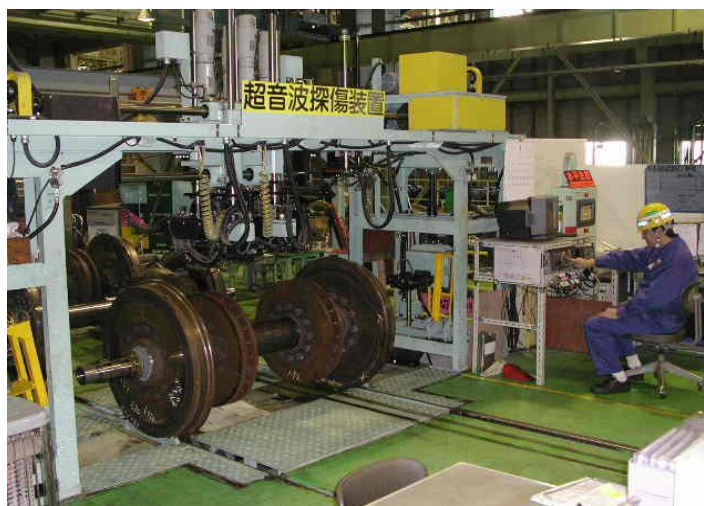
Ultrasonic inspection of axles
