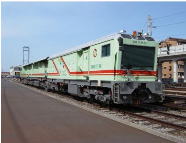
Rail grinding machines
