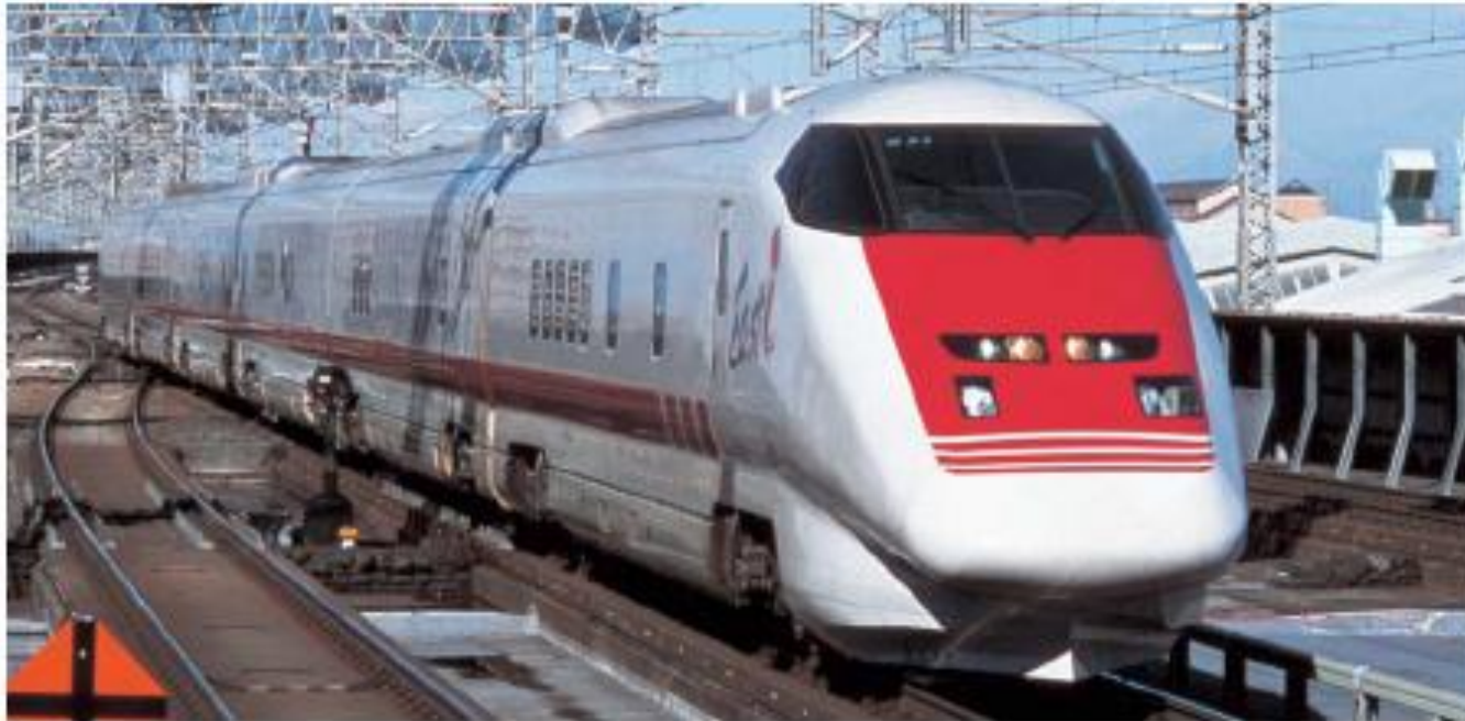
East-i (Shinkansen electric equipment and track inspection car)
